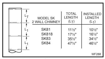
Fig. 7 Installed lengths of chimney sections.
